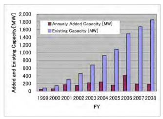
Figure 4 Wind Power Capacity, Added and Existing (JWPA)
